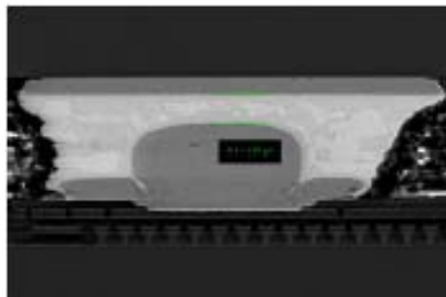
Cubic Wafer , die-to-wafer, 25um pitch
